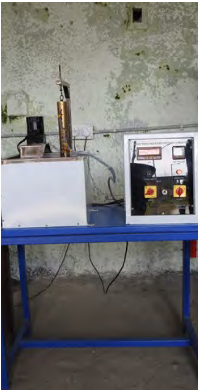
Fig: Study of steady and unsteady state heat conduction apparatus
