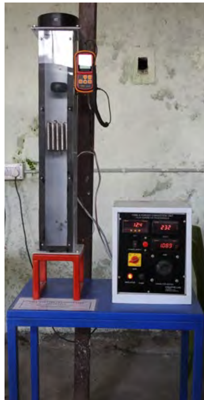
Fig: Free and forced convection apparatus can be fitted with fins.
