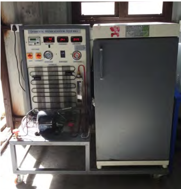
Fig: VCR test rig (domestic refrigerator)-manual mode
