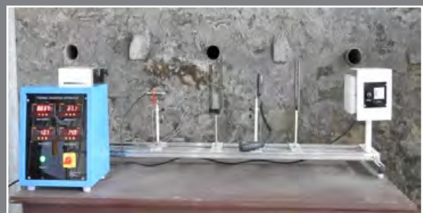
Radiation Apparatus with Radiation Shield Arrangement
