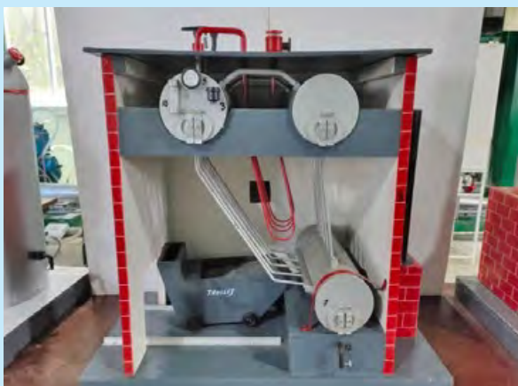
Cut-section model of Stirling boiler
