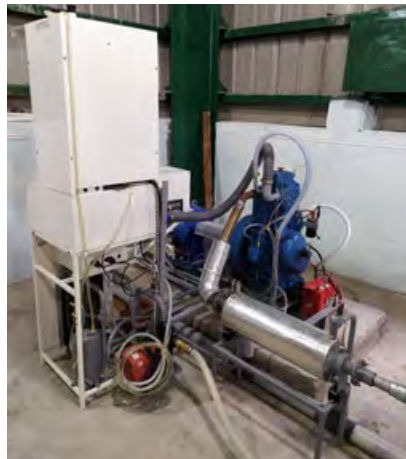
Fig:VCR multi fuel engine test Rig with variable test facilities & digital panel (ECU)
