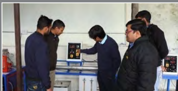
Heat Exchanger with Parallel Flow and Counter Flow Arrangement
