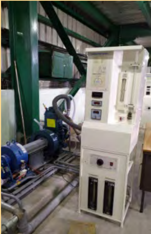
Fig: Diesel engine test Rig with variable test facilities and digital panel
