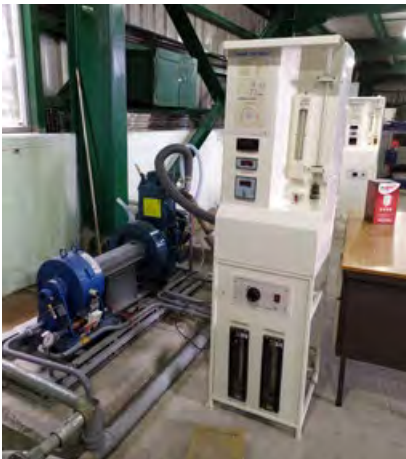
Fig: Diesel engine test Rig with variable test facilities & digital panel
