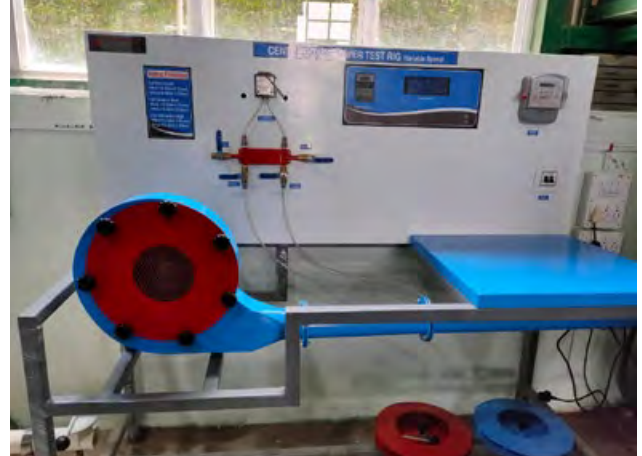
Fig: Centrifugal blower with data logging facility
