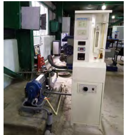
Fig: Petrol engine test Rig with variable test facilities & digital panel
