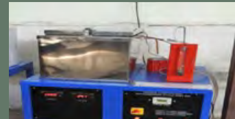
VCR test rig (ice plant)-computerized mode
