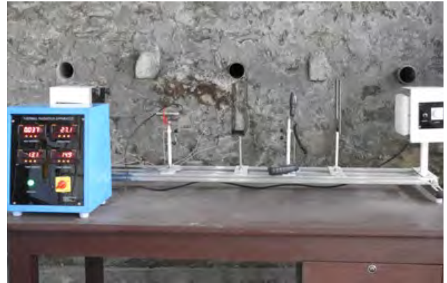
Fig: Radiation apparatus with radiation shield arrangement.
