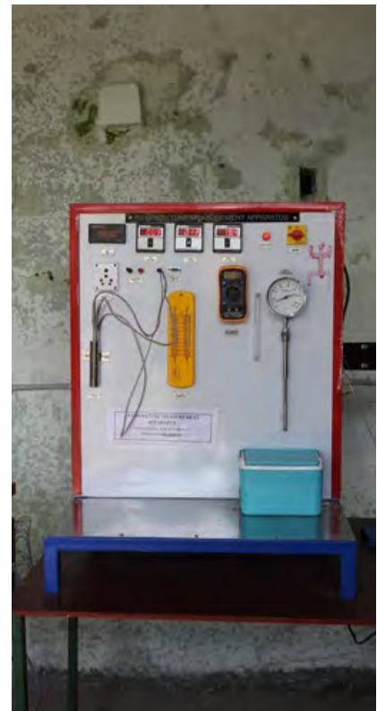
Fig: Temperature measurement module with several test methods.
