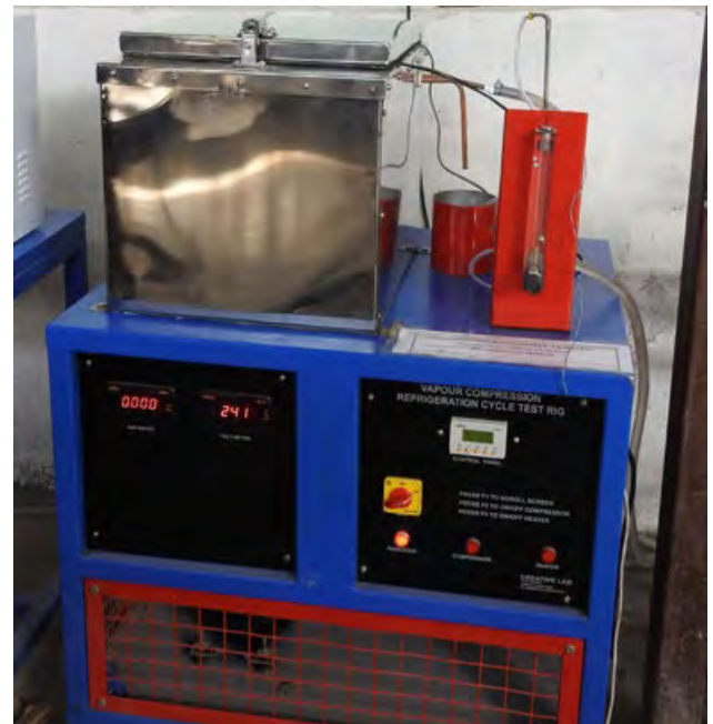
Fig: VCR test rig (ice plant)-computerized mode
