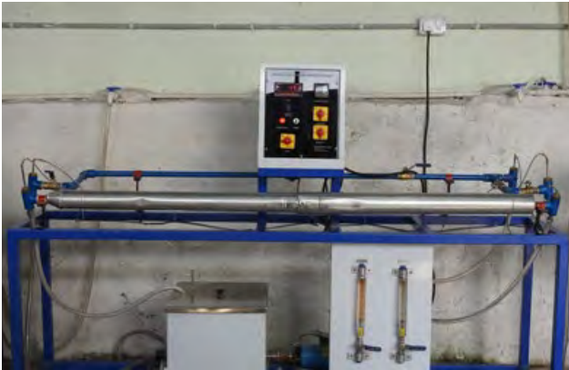
Fig: Heat Exchanger with parallel flow and counter flow arrangement
