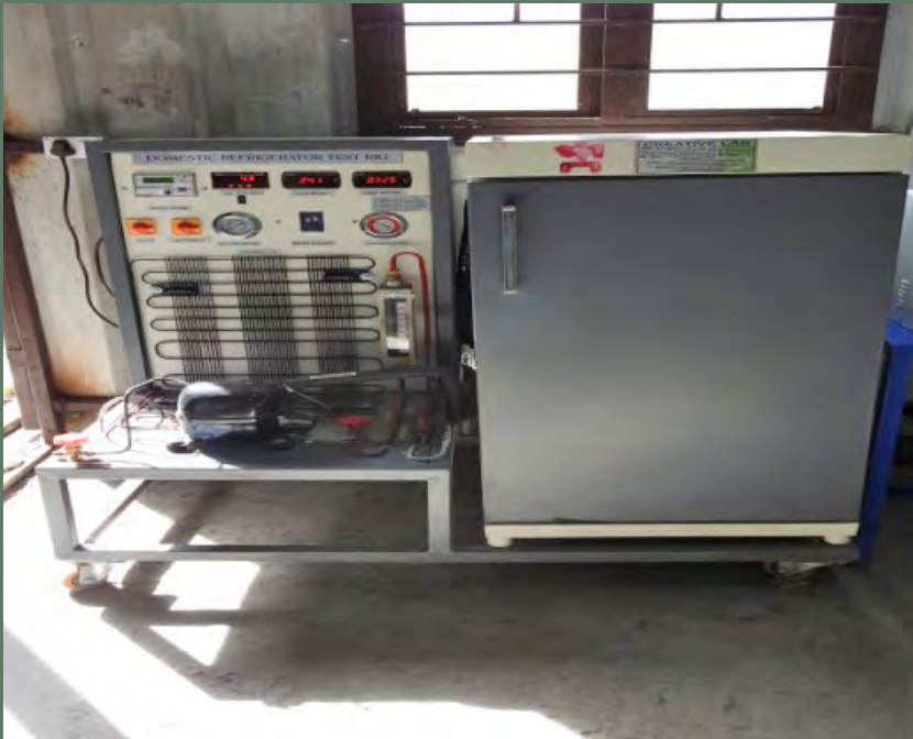
VCR test rig (domestic refrigerator)-manual mode
