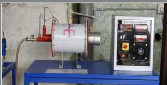
Determination of thermal conductivity of metal rod apparatus
