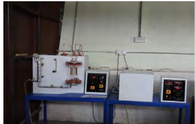
Fig: Boiling phenomena observation and thermal conductivity measurement of liquids apparatus.
