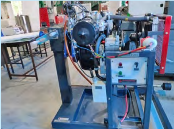
Assembling and dismantling set-up of 4-S 4-C petrol engine (working)
