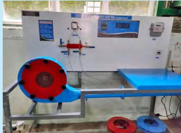
Centrifugal blower with data logging facility
