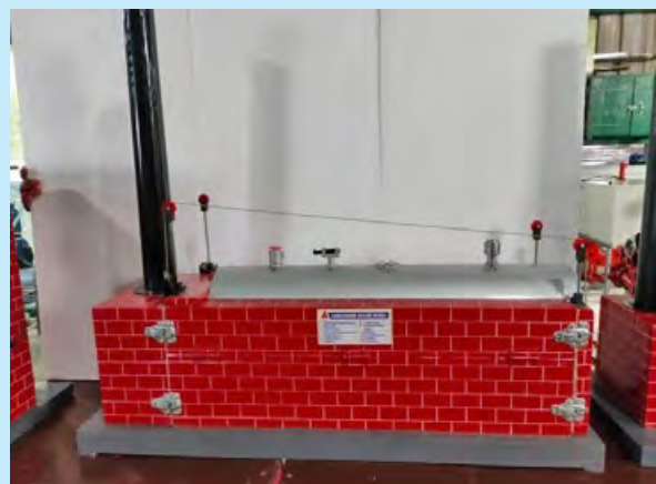
Cut-section model of Lancashire boiler
